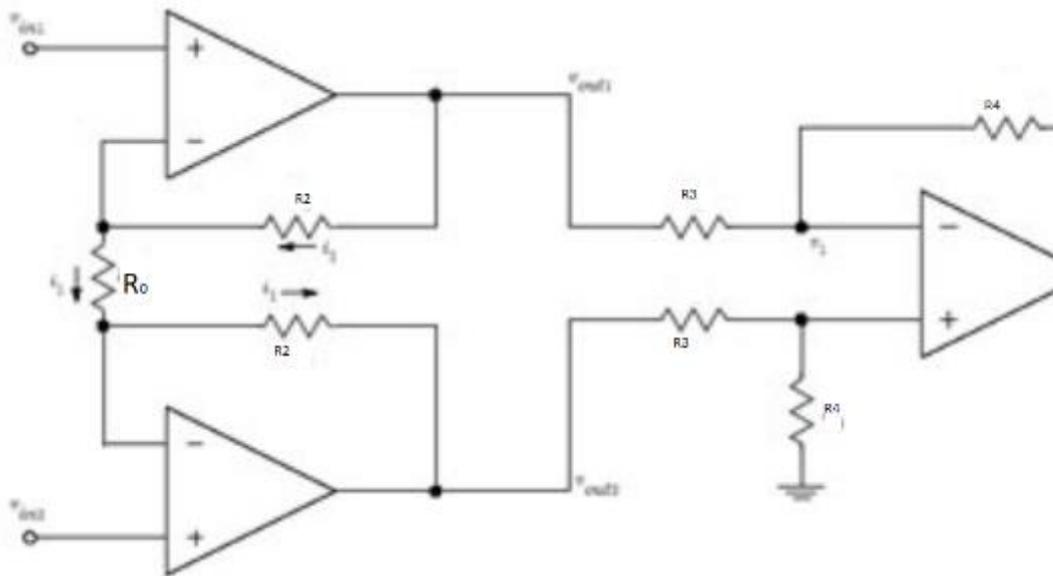
$$10 = \left(1 + \frac{20k\Omega}{R_0}\right) \cdot \frac{10k\Omega}{10k\Omega}$$
